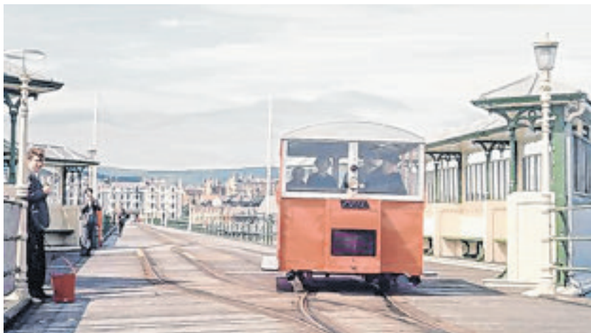
A 1950s view of the Wickham trolley taking passengers along the 3ft gauge pier railway at Ramsey
