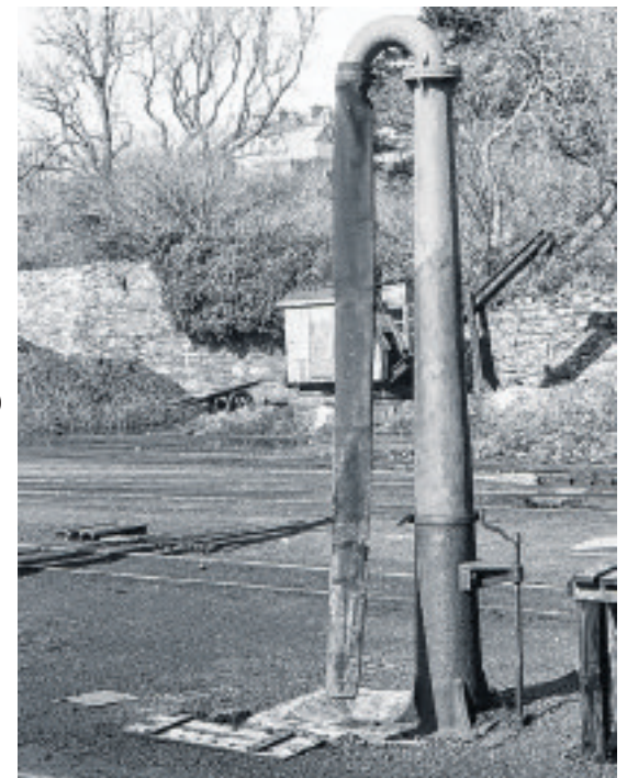
An original water crane or column which is still in use at Douglas station (Picture above and left: John Maddrell)
