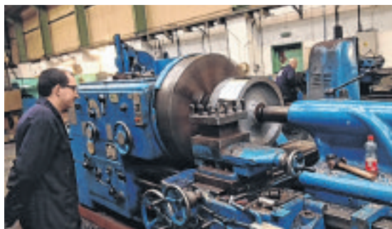
Machining one of the bearing rollers to take a new steel 'tyre' in 2013
