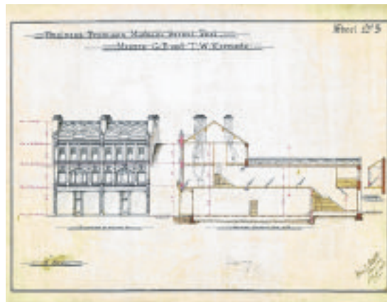
JJ Boyd's plans for Kermode's new premises (now Paradise and Gell) showing not only the façade which is still intact, but also how much more there is behind the street line
