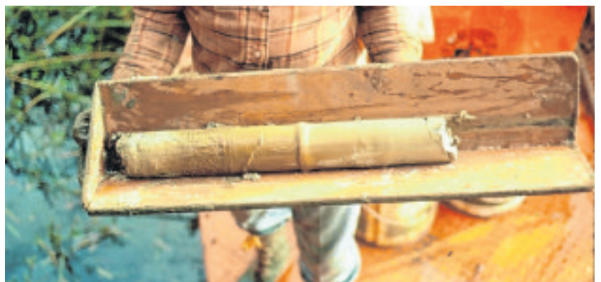
(Below) Trays are used to collect the cores, some of which – when drilling through glacial till / boulder clay – are quite fragile. (Above) A section of the 4-inch drill core from the test bore below Knock-e-Dhooney
