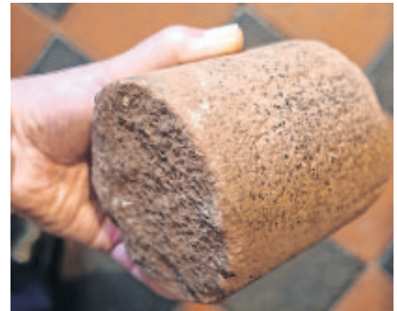
(Below) Trays are used to collect the cores, some of which – when drilling through glacial till / boulder clay – are quite fragile. (Above) A section of the 4-inch drill core from the test bore below Knock-e-Dhooney
