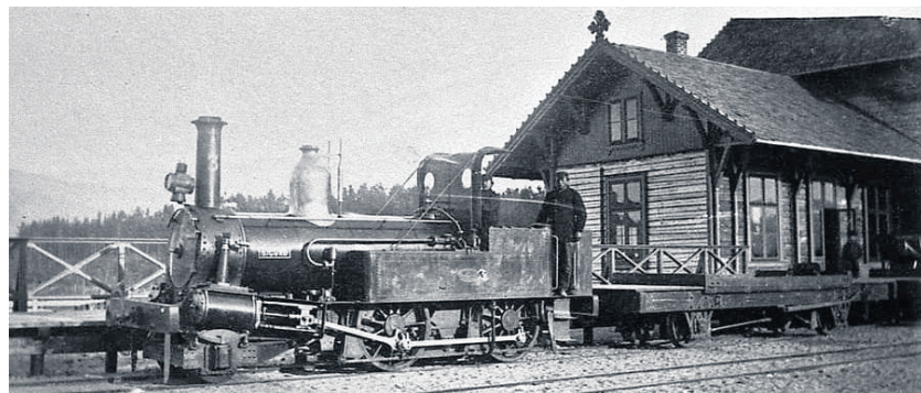
A Norwegian Government Railways Beyer Peacock locomotive of similar design to the Isle of Man Railway engines, No 3 Sigurd, stands at a wayside station in the early days of Carl Abraham Pihl's narrow gauge lines
